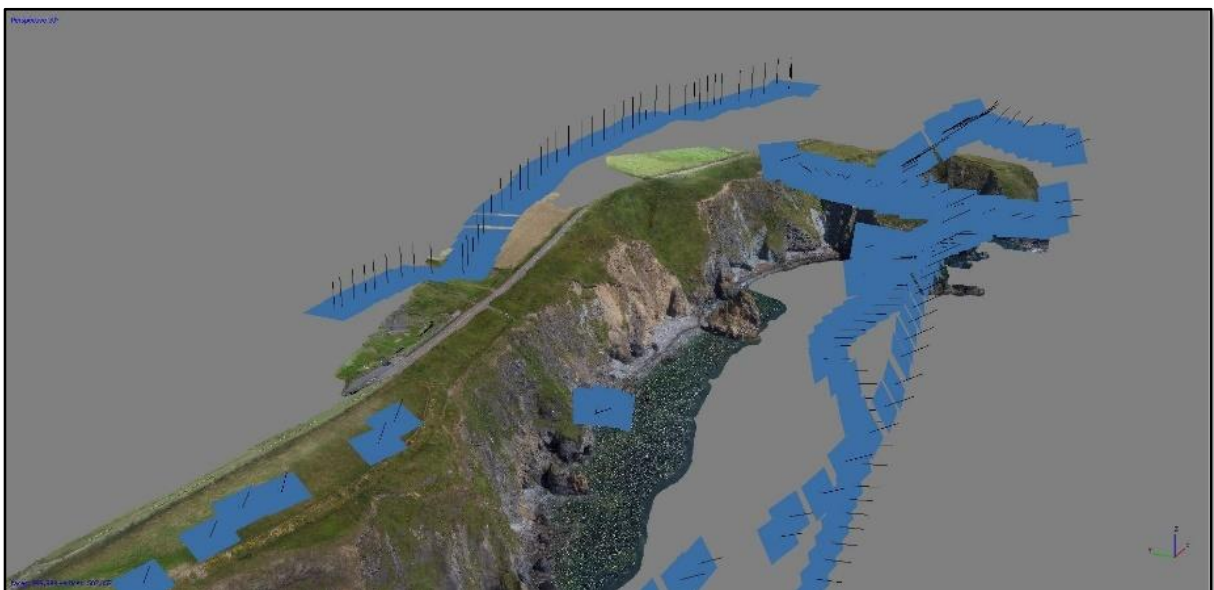
Figure 5. Snapshot of 3D model processing with image positions plotted in 3D space.
