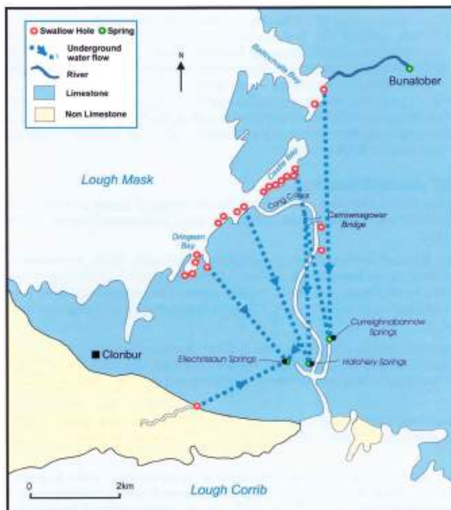
The Cong Canal and underground flow routes for water between Loughs Mask and Corrib (David Drew)
