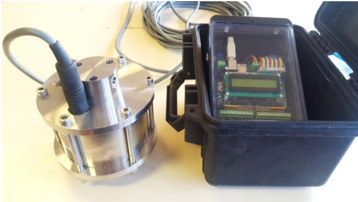
Figure 4 Field fluorometer and data logger in double waterproof housing
