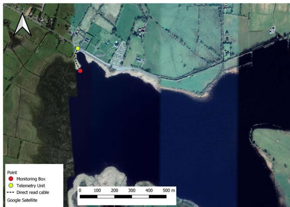
Figure 2: Monitoring equipment site map, Glenamaddy Turlough, Co. Galway
