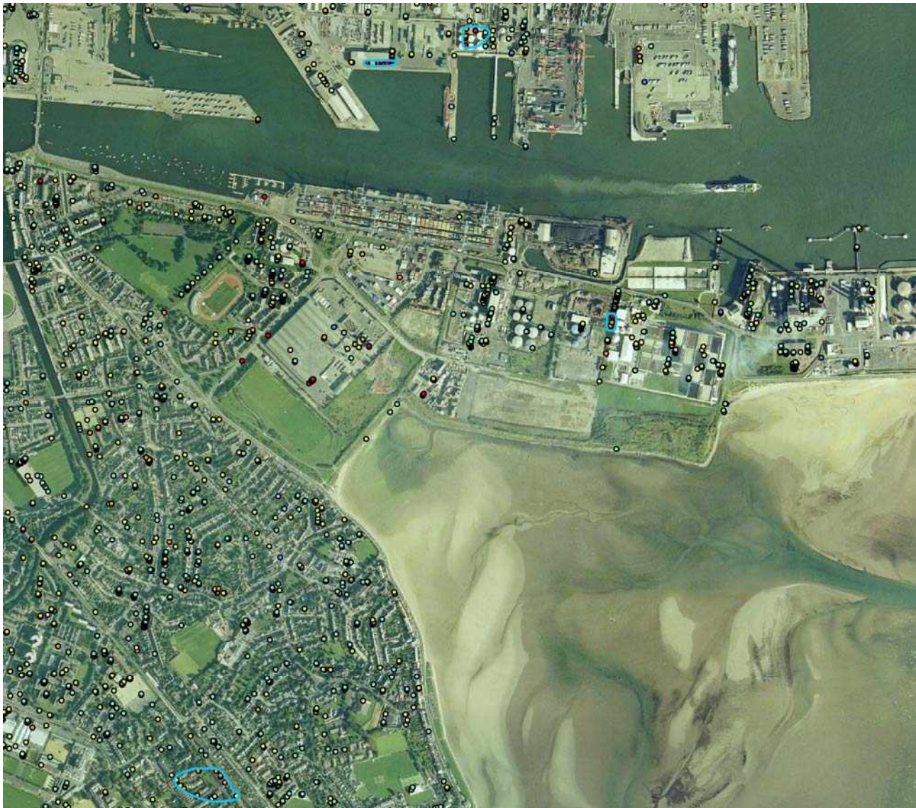
Fig PGGH_Dublin_002.2 Distribution of anthropogenic subsidence polygon (blue outline) and ERS PSI point data (red & orange indicate movement away from the satellite) on aerial imagery (Licence No. EN 0047212).
