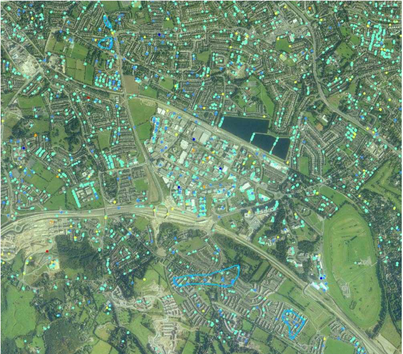
Fig PGGH_Dublin_001.2 Distribution of uplift polygon (blue outline) and Envisat PSI point `data (blue indicates movement towards the satellite) on aerial imagery (Licence No. EN 0047212).
