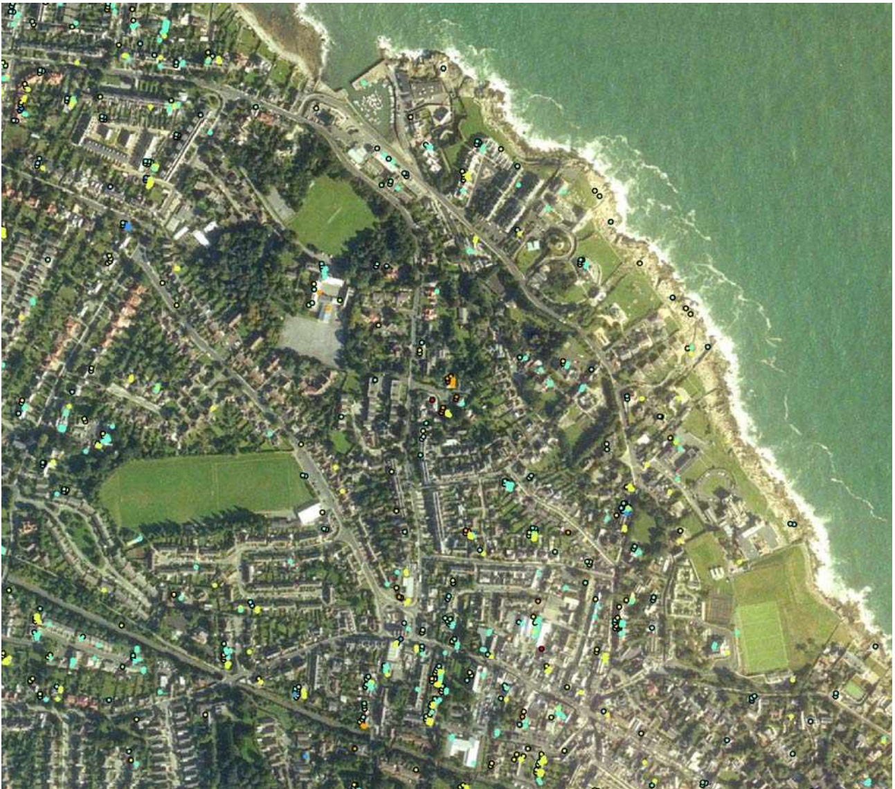
Fig PGGH_Dublin_005.2 Red and orange ERS points (with black outline) and Envisat PSI points (no outline) showing a confined area of subsidence (Licence No. EN 0047212).
