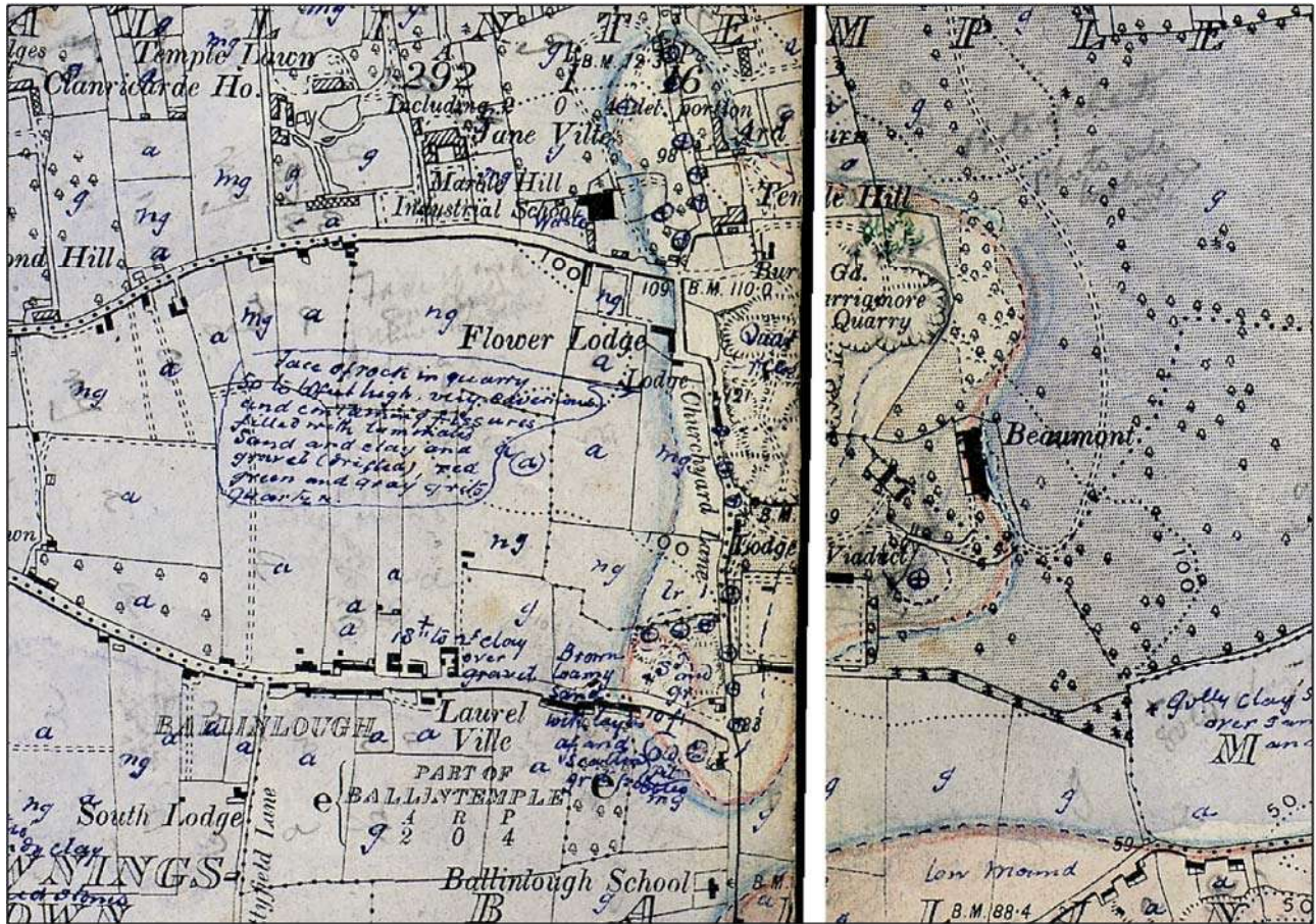
Fig PGGH_Cork_005.6 Ordnance Survey Ireland Historic 6 inch (1: 10,560) mapping (Licence No. EN 0047212) with Geological Survey of Ireland annotations describing the cliff face as "very cavernous and fissured."
