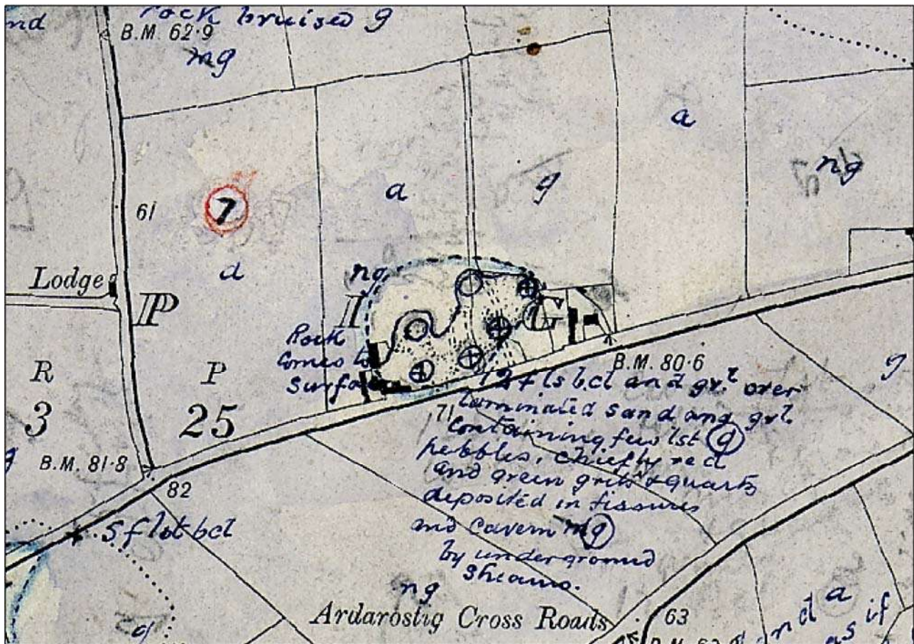
Fig PGGH_Cork_005.4 Ordnance Survey Ireland Historic 6 inch (1: 10,560) mapping (Licence No. EN 0047212) with Geological Survey of Ireland annotations detailing the presence of fissures and caverns typical of the area.
