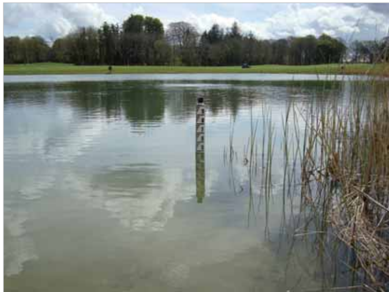
Figure 3-2: Water level monitoring in surface water body
