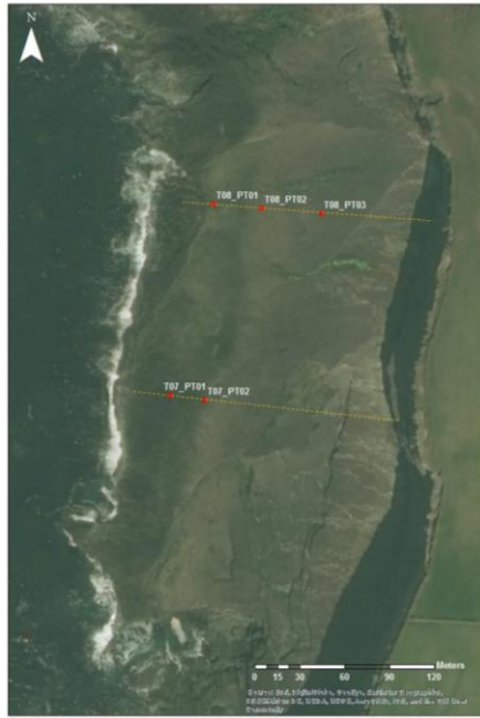
Figure 6. Topographic transects (yellow dashed lines) and the locations of pressure transducers (red dots) deployed at Ballard Bay Platform for August (T07_PT01 and T08_PT01) and November (T08_PT01, T08_PT03). Instruments deployed at other locations on this figure failed to return data.
