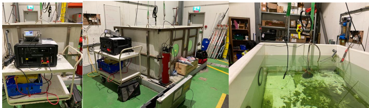
Figure 14. Testing of sound projector equipment at P&O Maritime, Galway, April 2023. (top left) DC-AC inverter (top right) Experiment overview, showing DC-AC inverter, iMARL ORCA, water tank and suspended hydrophone cable. (bottom) View of tank, showing submerged hydrophone, as well as the source transducer of the sound projector.
