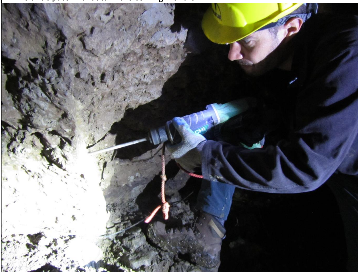
Figure 2. Project team member, Nick Scropton (Maynooth U.), sampling a flowstone in Doolin Cave for U-Th dating. This minimally invasive technique enables us to date the speleothem without causing visible damage to cave surfaces. U-Th ages from speleothems afford the minimum-limiting age control for calibrating nuclide production.
