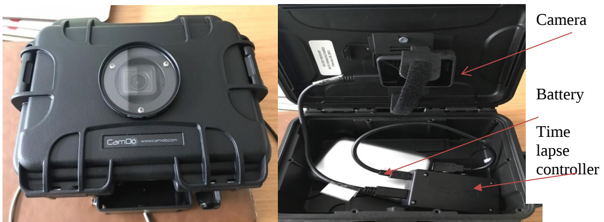
Fig. 3 Weather proof camera box with camera, battery and time lapse controller
