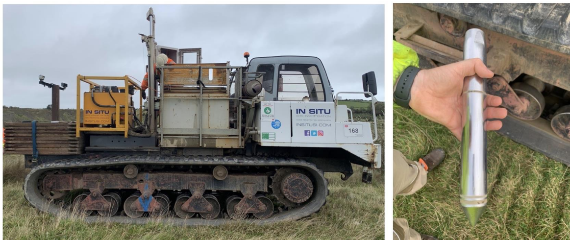
Figure 5: (a) CPT rig and (b) CPT cone used for site 3 ground investigation (from Gallagher 2022)
