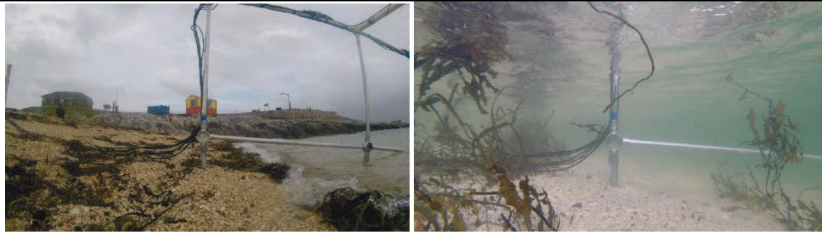
Figure 9 (left): The GoPro video mounted at the side of the frame was able to capture the intrawave sediment transport to additionally be a visual check for the distance sensor data. Figure 10 (right): Example of immersed GoPro footage.
