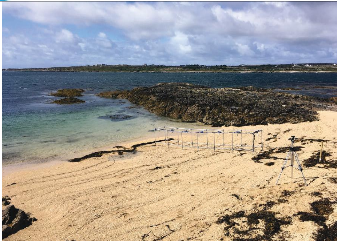
Figure 5: The frame with seven ultrasonic distance sensors mounted to monitor the morphodynamic response with the incoming and outgoing tide and the intrawave sediment transport.
