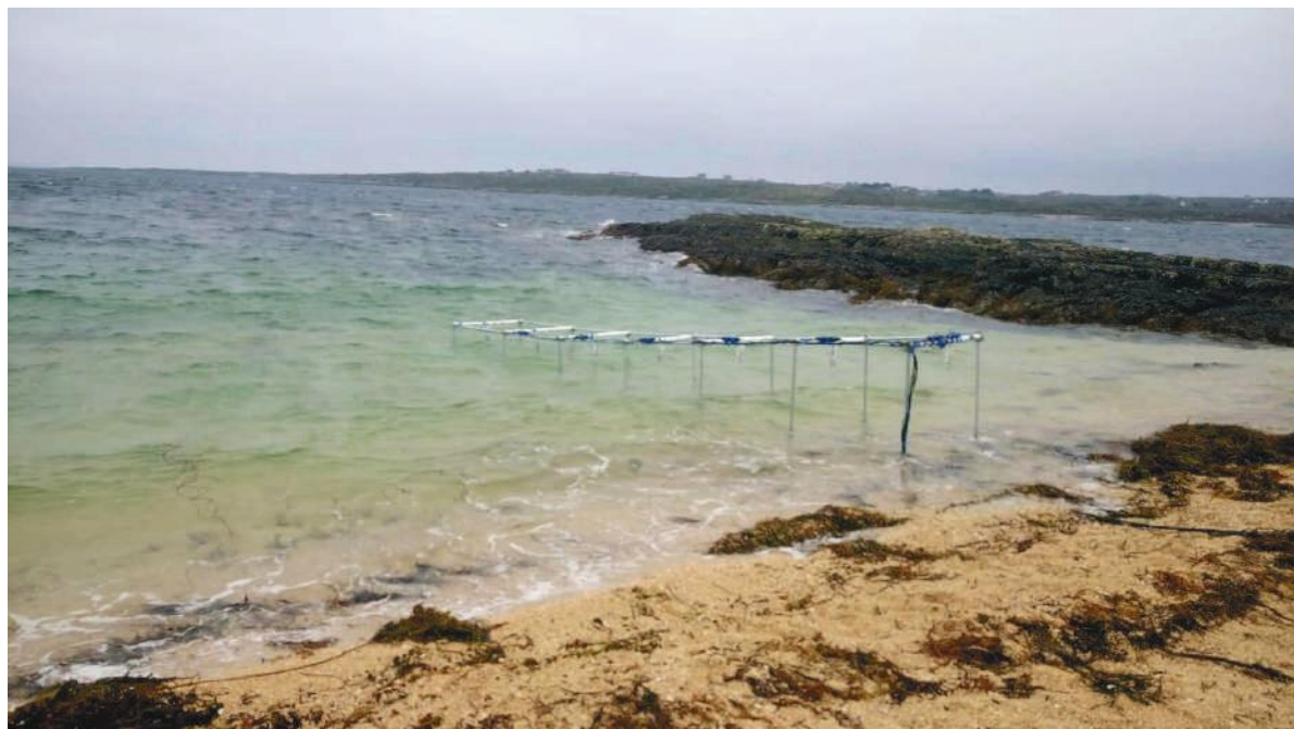
Figure 6: The frame needed to be strong enough to withstand the flooding (and ebbing) tide.
