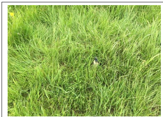
Figure 9: Installed soil water suction samplers (centre of photographs) at the tillage and grass-land (perennial ryegrass) sites at UCD Lyons Research Farm (Newcastle, Co. Dublin). For much of the summer these sites suffered substantial soil moisture deficits and sampling of soil pore waters was not possible. At the time of writing (November 2018), deficits are close to zero and soil pore-water sampling has recommenced. Geochemical results from the Feighcullen site in Co. Kildare are more complete as summer moisture deficits were less severe compared to the Lyons and Killinthomas sites.
