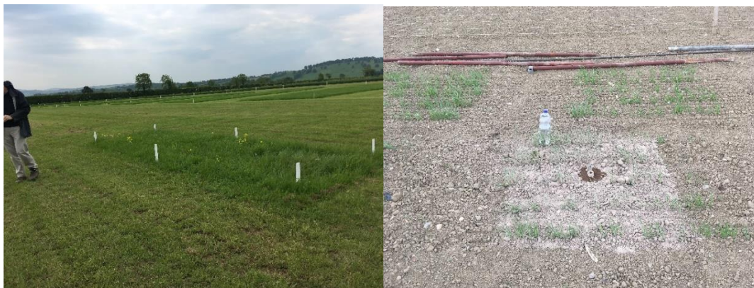
Figure 1. Overview of experimental sites at UCD Lyons Research Farm (A) grass soil and (B) crop soil immediately after finely crushed basalt was spread. The soil-water suction sampler is visible near the centre of the treated area. Shallow soil samples were also taken from these sites for the laboratory experiments described below.
