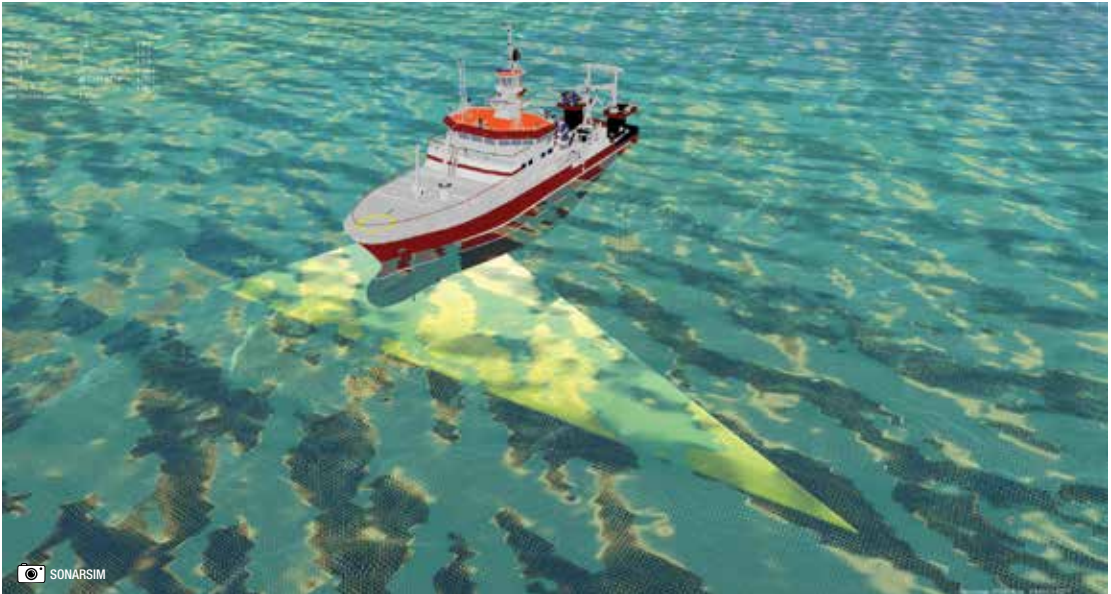
Figure 1: Simulation scenarios with immersive transparent ocean rendering of vessel motion, seabed geometry/sediment classification, sonar footprints, sea surface swell, etc. enhance situational awareness and improve cause and effect feedback through visual cues.
