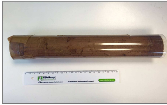
Figure 5: 30x4cm Soil sample encased in plastic lining
