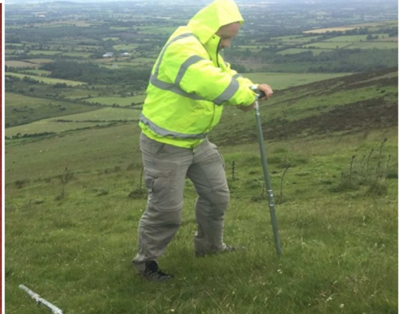
Figure 4 Soil auger (left) and use in field (right)
