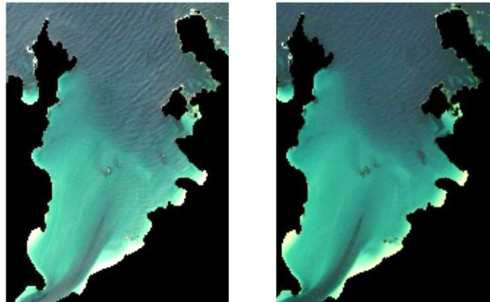
Figure 5: Water should absorb any NIR energy before it returns from the sea-floor, so any NIR energy measured is assumed as coming from sun-glint and can be used to remove this contribution from other bands (a) a Sentinel 2a image of Mulroy bay before correction – wave motion (which generally reflects back toward the sensor) is visible (b) after correction sunglint has been successfully removed.
