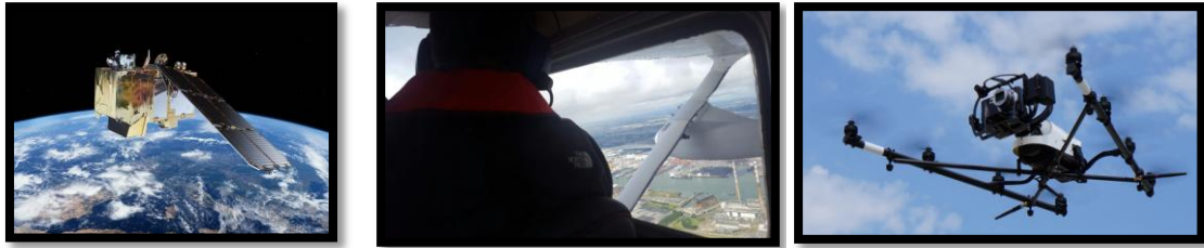
Figure 2: The multiresolution approach to deriving bathymetry (a) imagery from satellite incorporates high quality sensors and regular image updates but result in a large measurement range (b) light aircraft reduce range to target and increase resolution but are not quick to mobilise (c) drones operate on-demand at low altitude, providing high resolution images but limited by regulations and payload.
