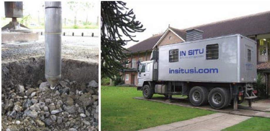
Figure 30 CPT testing ( http://www.insituser.com/research/ ).
