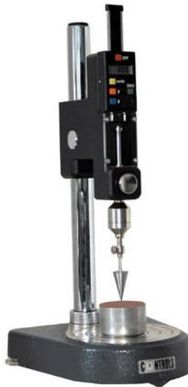
Figure 40 An exaple of Liquid Limit cone penetration method ( http://www.sisc.com.vn/en/detail.php?module=product&iCat=2097&iData=221&#page=page-3 ).
