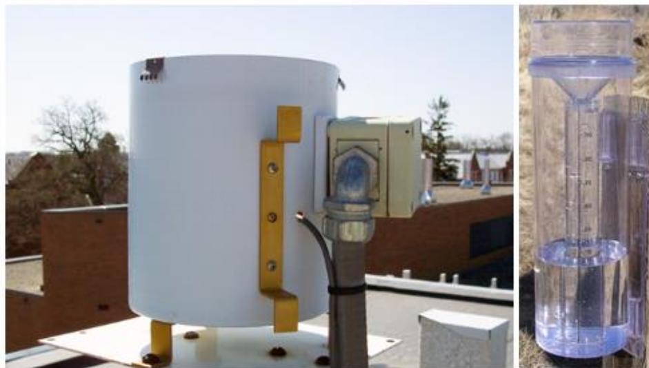
Figure 42 Optical gauge (automated system) and standard type rain gauge (required direct readings) ( http://www.nwclimate.org/guides/how-to-use-rain-gauge/ ).
