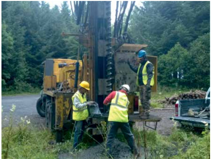
Xavier Pellicer (left) sampling till in Glenfarne, Co. Leitrim, using the GSI Drill Rig in auger mode with drillers Ger Cott (centre) and Oisín O'Brien
