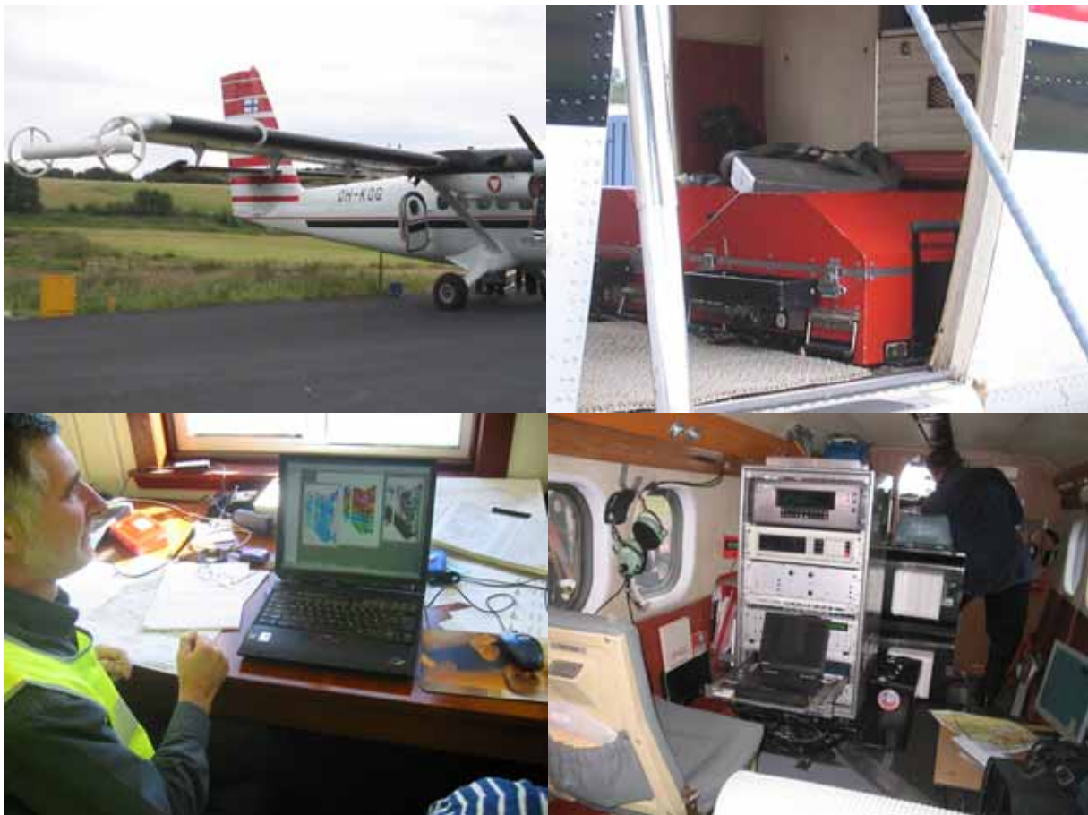
Clockwise from top left: the magnetic and electromagnetic sensors on the wing tip of the aircraft; the radiometric sensors inside the aircraft; recording and operations inside the aircraft; and post survey processing.
